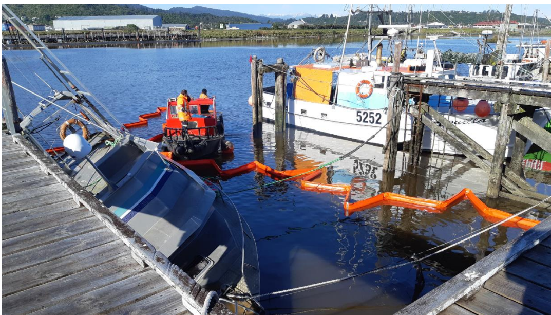
Figure 2: Rapid deployment boom being deployed 29-06-2021:
