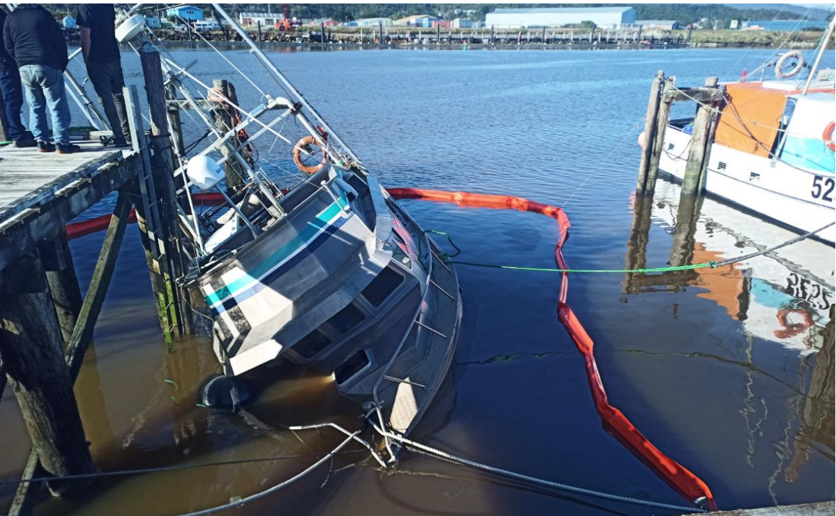
Figure 4: Vessel contained within boom:
